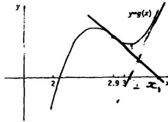
As 2.9 is on the opposite side of the stationary point to the root, the tangent will cut the x-axis further from the root than the original approximation. (2)
